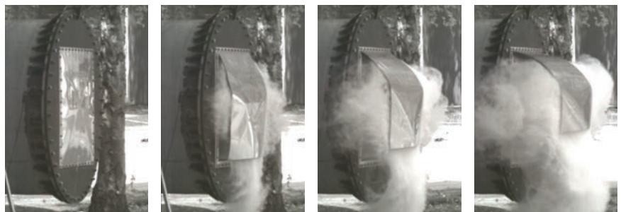
Explosion test on vent panel
