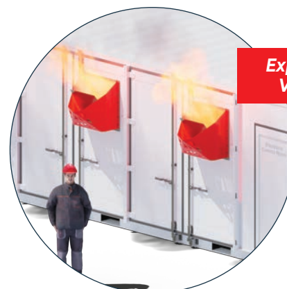
Explosion without VIGISPACE®
