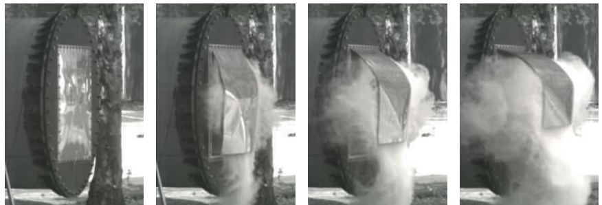
Explosion test on vent panel
